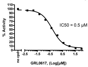
Inhibition of PLPro Protease enzyme activity by GRL0617, measured using the *Papain-like Protease Assay Kit: Protease Activity (BPS Bioscience #79995-2).* Fluorescence intensity was measured using a Tecan fluorescent microplate reader. *Data shown is lot-specific. For lot-specific information, please contact BPS Bioscience, Inc. at info@bpsbioscience.com*
