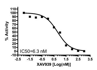
Inhibition of TNKS1 enzyme (Cat. # 80504) with XAV939 (Cat. # 27100), measured using the TNKS1 Histone Ribosylation Assay Kit (Biotin-labeled NAD+), BPS Bioscience (Cat. # 80579). Luminescence was measured using a Bio-Tek fluorescent microplate reader. *Data shown is lot-specific. For lot-specific information, please contact BPS Bioscience, Inc. at info@bpsbioscience.com*
