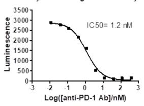
Inhibition of PD-1-PD-L1 binding by PD-1 Neutralizing Antibody (BPS Bioscience, #71120). Luminescence was measured using a Bio-Tek fluorescent microplate reader. *Data shown is lot-specific. For lot-specific information, please contact BPS Bioscience, Inc. at info@bpsbioscience.com.*
